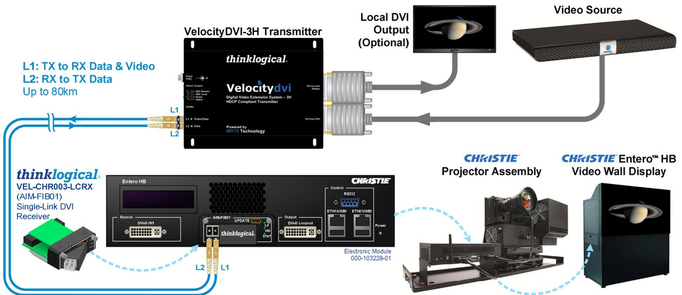
For simple plug-and-play, the system requires two fibers; one for video transmission (L1) and one for EDID table support (L2). Single fiber applications (fiber L1, TX to RX only) require that the Christie EDID table be manually loaded into Thinklogical's transmitter for support of the Christie resolutions.
